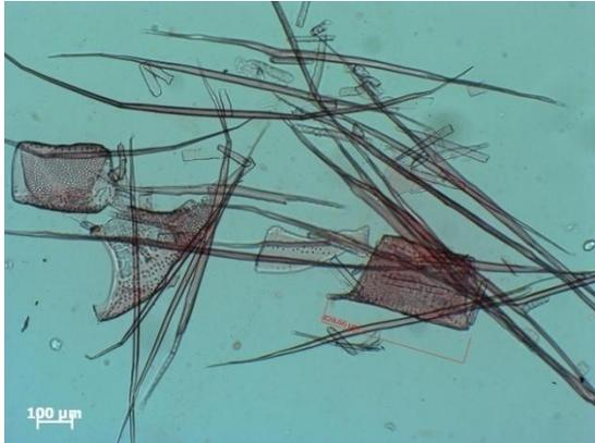
Figure 1 Fiber and vessel of meranti sangkan (40 x).
