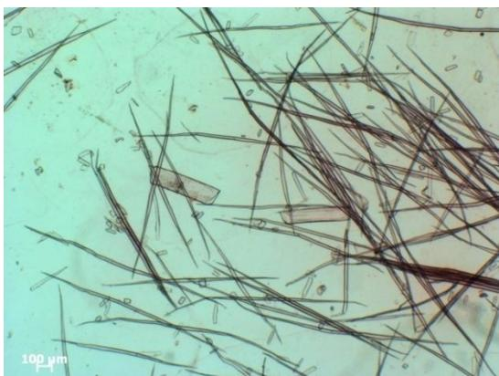
Figure 3 Fiber and vessel of meranti bunga kulit hitam (10x).
