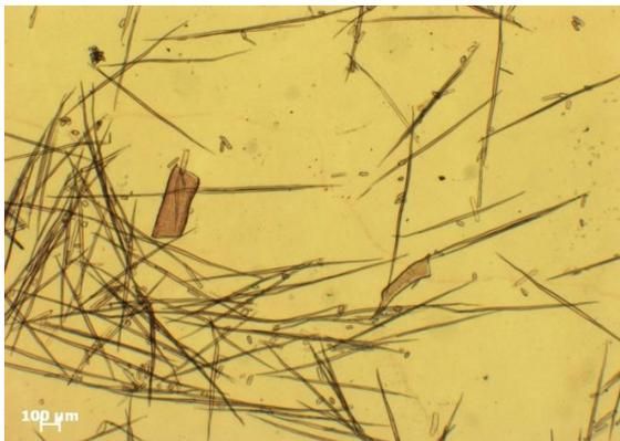
Figure 2 Fiber and vessel of meranti bakau (10x).
