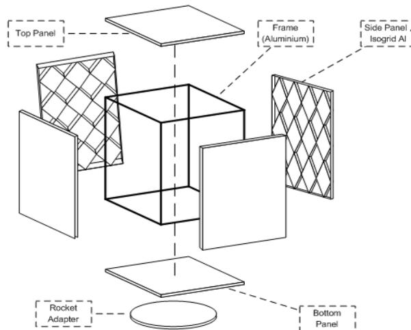
Figure 3-2: Lay out the structure concept of G2-SAT<sup>1</sup>
