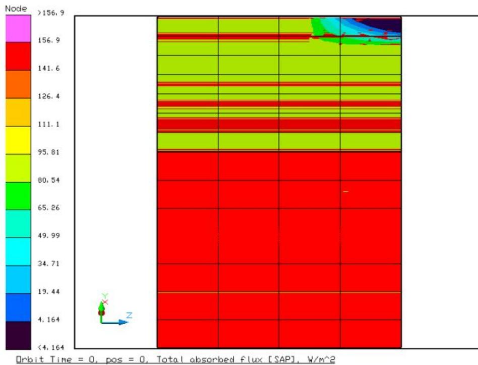
Figure 4-3B: Orbital heating rates case 2 from back-right view
