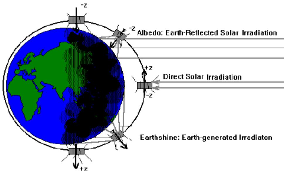
Figure 2-2: Three primary terms of the heat loads for calculating G2-SAT orbital heating rates
