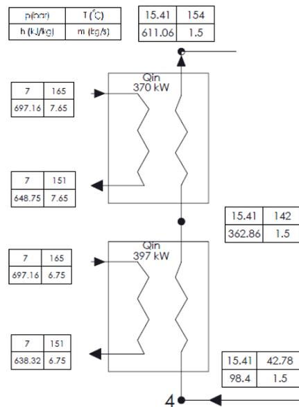
Figure 4 . Thermal balance of heat input
