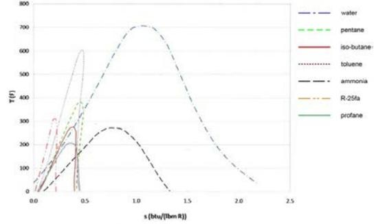
Figure 2 T-s Diagram for several kind of fluid
