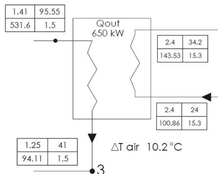
Figure 5. Thermal balance of condenser
