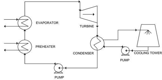
Figure 3 ORC Schematic Diagram
