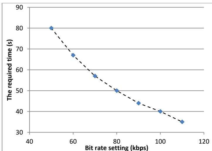
Figure 7. The time for sending a single image
