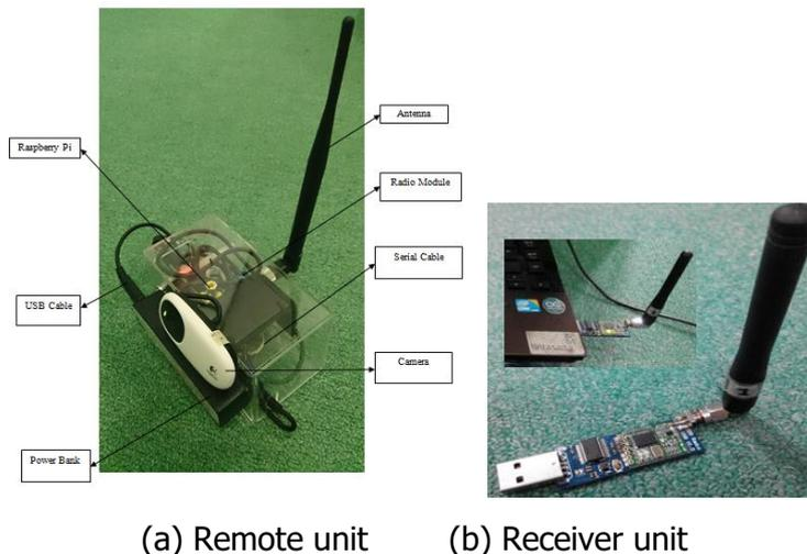
**Figure 2.** The evaluated 433 MHz radio system
