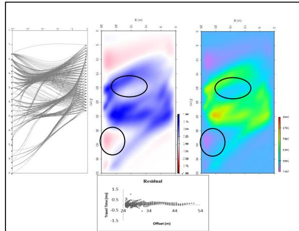
Figure 3. Inversion results of BH2A-BH1. Top Left to right: ray paths from sources to receivers through final model, perturbed final velocity model, and absolute final velocity model. Bottom: residual travel times between observed travel times and calculated travel times.
