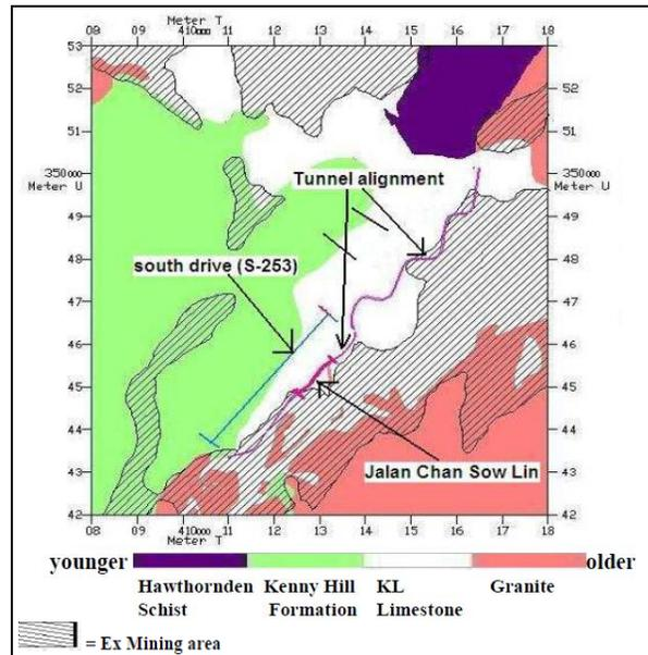
Figure 1. The geological map around the tunnel alignment (left) and a cross section through this area (right). The alignment traverses through almost 100% the Kuala Lumpur Limestone formation.
