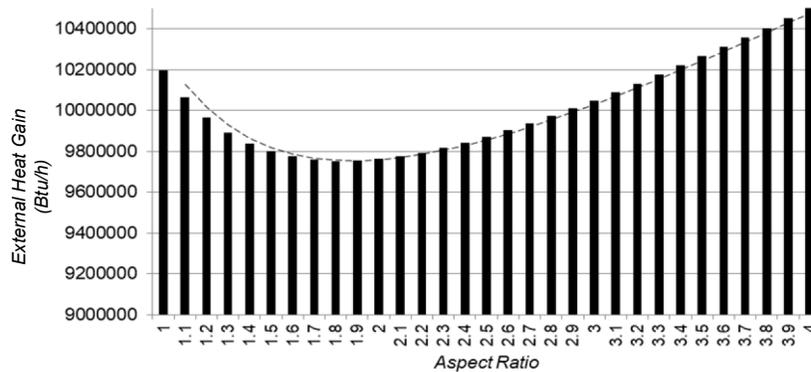
Figure 1. The correlation graph between aspect ratio and building external heat gain.
