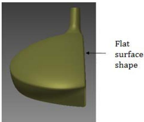
Figure 8. The head of the stick with the shape of the batter surface is designed flat
