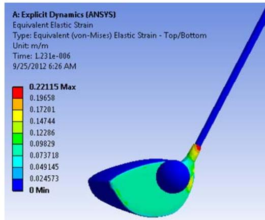
Figure 12. Strain distribution results from numerical simulations
