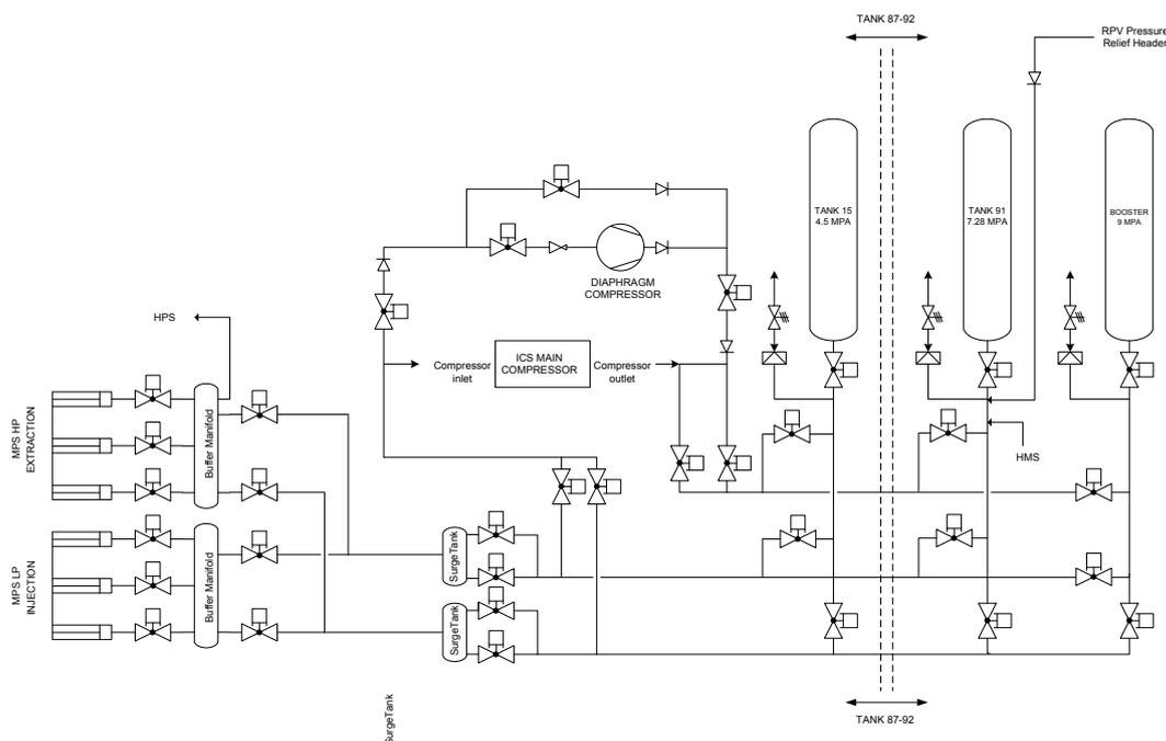
Fig. 1. ICS conceptual design of RGTT200K<sup>[10]</sup>
