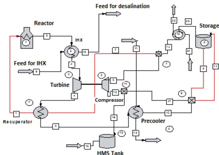
Fig. 4. The ICS model using ChemCAD
