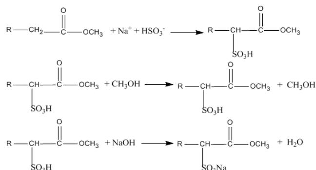
Figure 3. Reaction mechanism of methyl ester sulfonate formation
