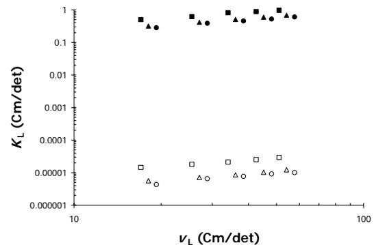
Figure 2. Overall Mass Transfer Coefficients,  $K_L$ , Under Various Number of Membrane Fibers in the Contactor of (■) 12, (▲) 15 and (●) 18 using DEA Solution as Absorbent, and (□) 12, (Δ) 15 and (○) 18 using Water as Absorbent
