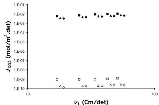
Figure 3. Fluxes of  $CO_2$ ,  $J_{CO_2}$ , under Various Number of Membrane Fibers in the Contactor of (■) 12, (▲) 15 and (●) 18 using DEA Solution as Absorbent, and (□) 12, (Δ) 15 and (○) 18 using Water as Absorbent
