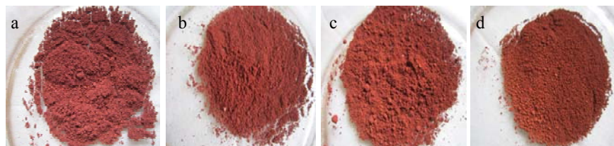
Figure 2. The color of hematite pigment synthesized at pH 6 (a), 7 (b), 8 (c), and 9 (d)
