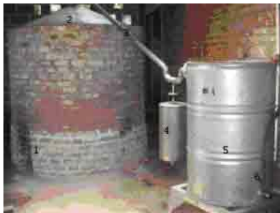
Figure 1. The home-scale convensional apparatus for pyrolysis: 1. Convensional furnace with wood as fuel; 2. Reactor; 3. Smoke flow pipe; 4. Tar condensed collecting; 5. Condenser; 6. Liquid smoke collecting.
