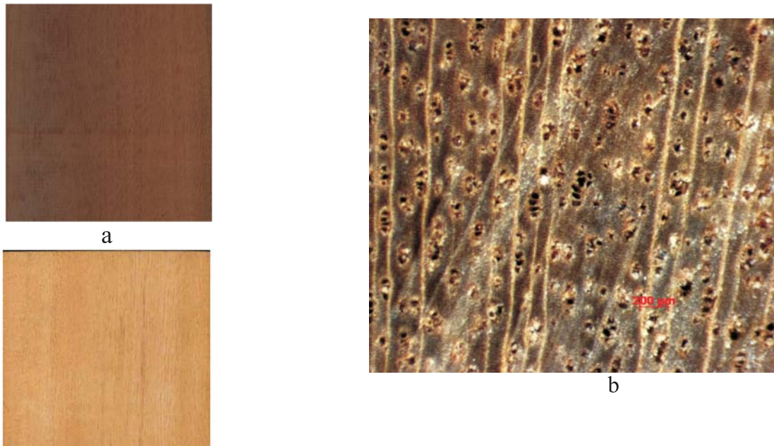
Gambar 9. Penampang memanjang (a) dan melintang (b) (makroskopis) kayu Olearia sp. 10x Figure 9. Longitudinal (a) and transversal (b) section of Olearia sp. in macroscopic feature, x10)
