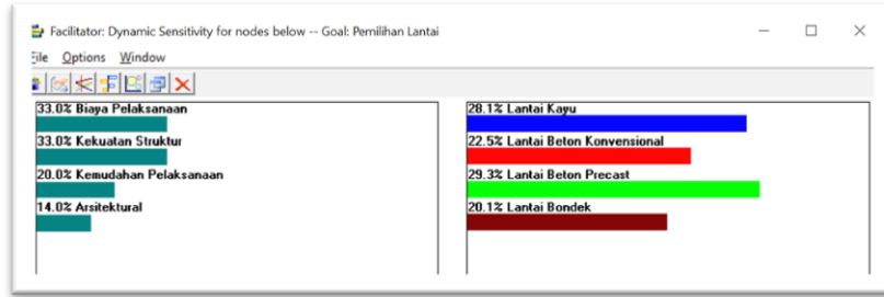
Gambar 7 Output Dynamic Graphic Synthesis
