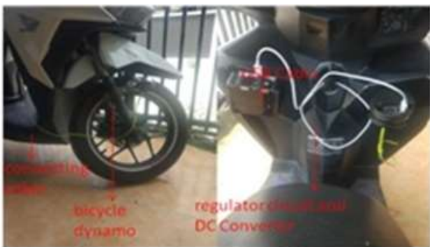
Figure 6: Installation of a circuit on a motorcycle
