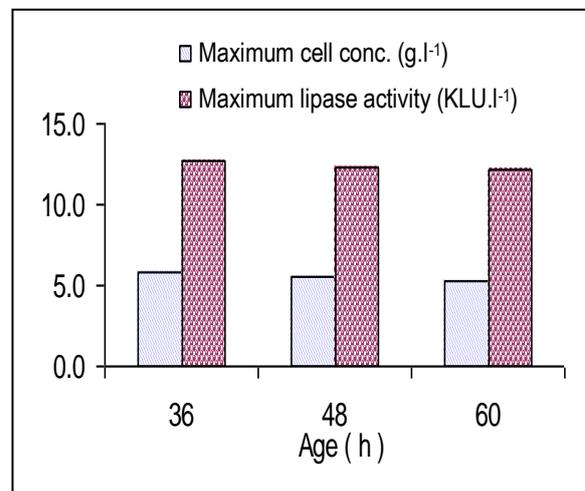
**Figure 7.** Effect of inoculum age on lipase production ( pH=6.0, T= 30° C, Aeration = 1 vvm, Agitation = 500 rpm and glucose = 10 g L<sup>-1</sup>)
