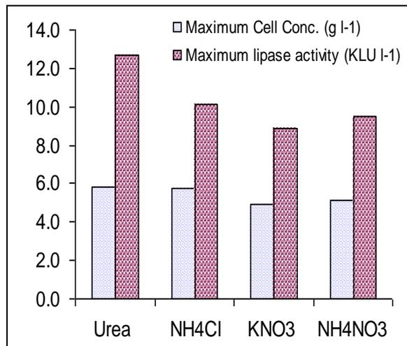
**Figure 6.** Effect of nitrogen sources on lipase production ( pH=6.0, T= 30° C, Aeration = 1 vvm, Agitation = 500 rpm and palm oil = 10 g L<sup>-1</sup>)
