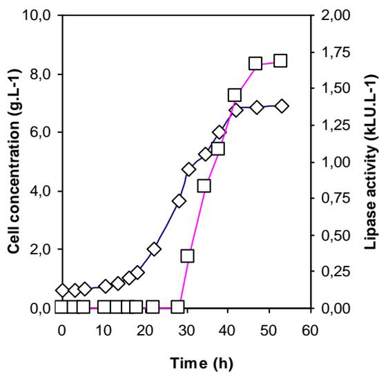
**Figure 4.** Profile of lipase production in 10 g L<sup>-1</sup> palm cooking oil ( pH=6.0, T= 30° C, Aeration = 1 vvm, Agitation = 500 rpm )
