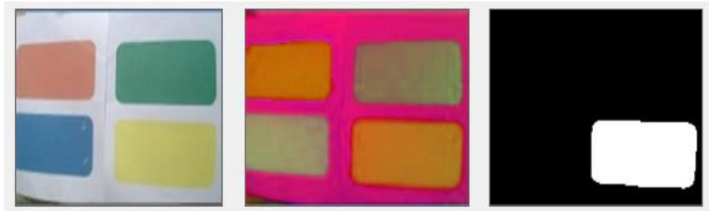
Figure 2. Yellow detection, from RGB to HSV to binary conversion
