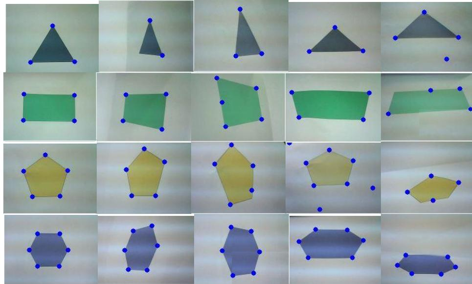
Figure 8. the test result of angle detection
