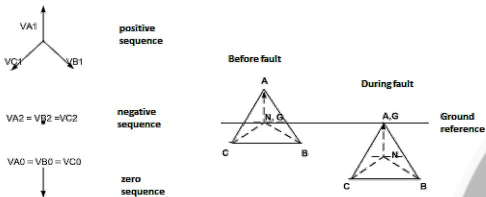
Figure 3. Ground Disturbance on Floating Grounding Systems
