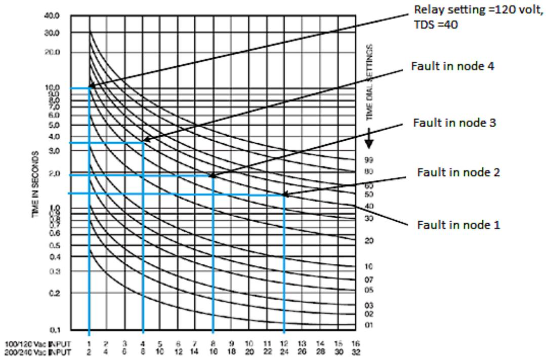
Figure 7 The Characteristic of The Overvoltage in Time of Inverse Termination
