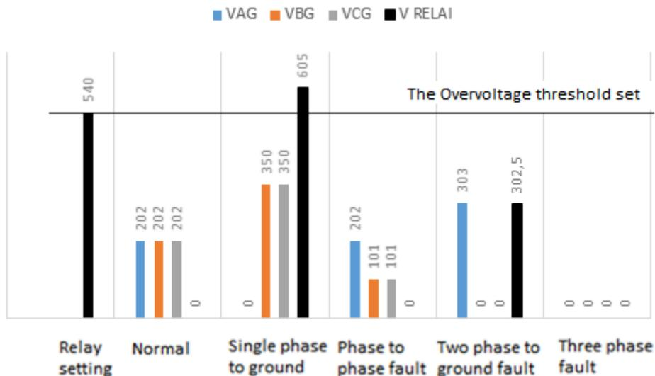
Figure 8 Voltage Function of Different Types of Disturbance
