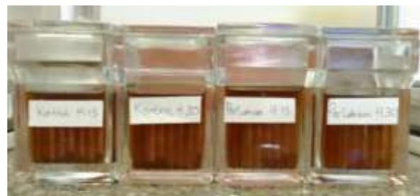
Figure 2. The coffee immersion of control and treatment group in the staining jar for 15 and 30 days
