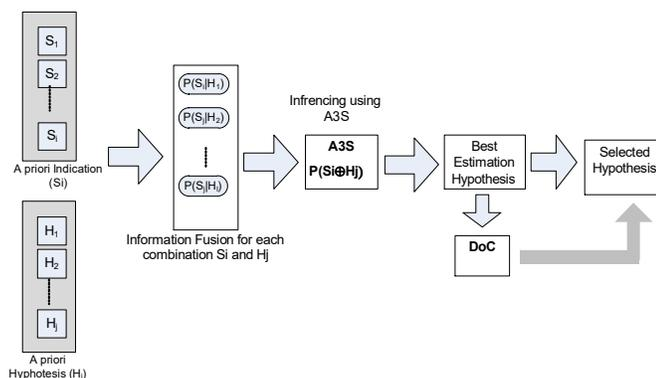
Figure 2. Mechanism to gain DoC value, started by fuse information from sensors and hypotesis [9]
