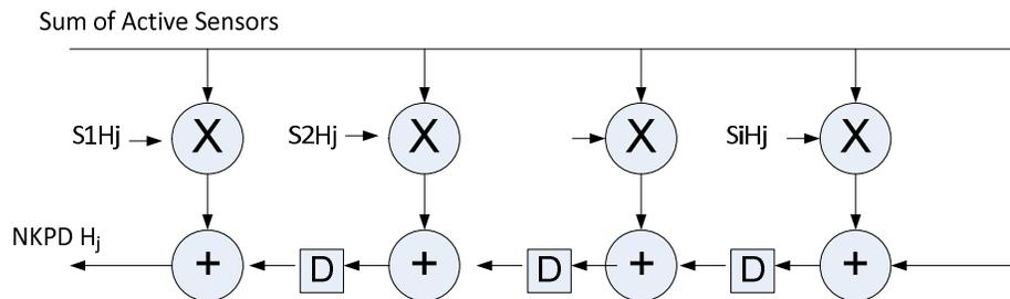
Figure 4. Systolic Array Processor of A3S computation
